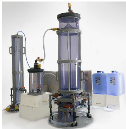
Figure 3 Picture showing the mini-SAFF bench scale unit, Primary, Secondary, and tertiary vessel and tanks.
