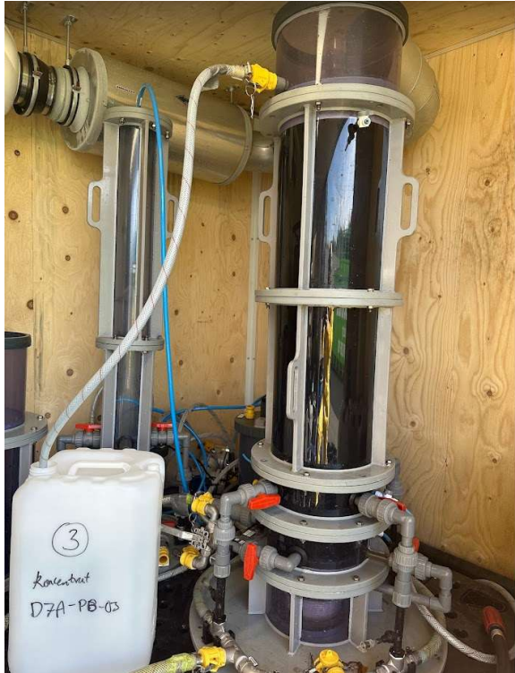
Figure 4 Photo of the bench scale SAFF filled to approx. 90% with untreated groundwater supplied by the client.
