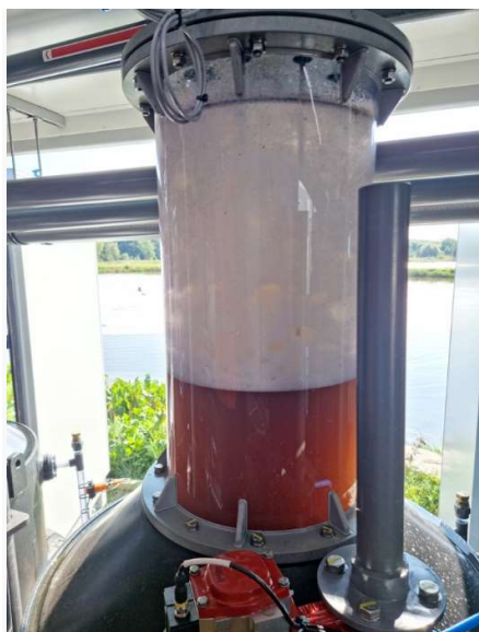
Figure 2 Photo taken during the second fractionation step in a full-scale plant. The dry foam can be seen being removed by vacuum.
