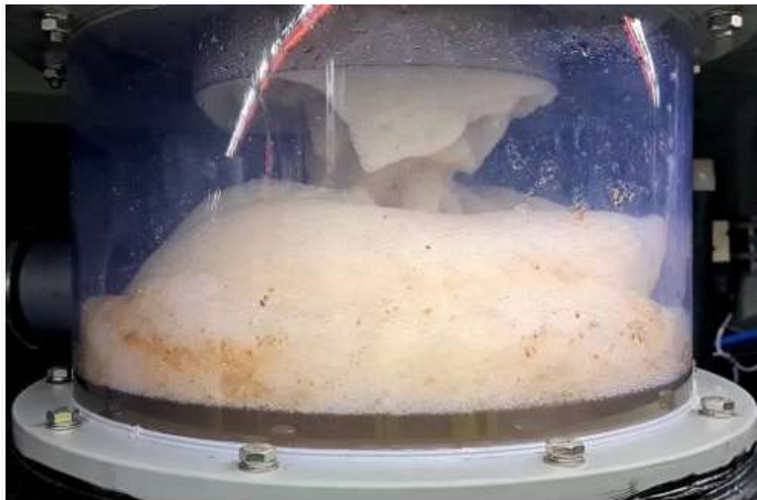
Figure 1 Photo taken during the execution of the first fractionation step in a full-scale plant. We see how in the first step you let foam “flow” over the edge of the centred inner tube in the column. You can also see the foam that accumulates during the separation and the top water where the less foam prone PFAS substances accumulate.
