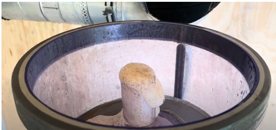
Figure 5 Separation of foam, spilling over the cone.
