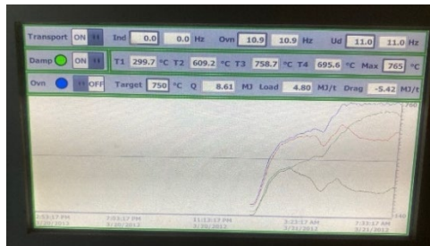
Figure 3: Temperature/time diagram of the activation of the wood-biochar at AquaGreen.
