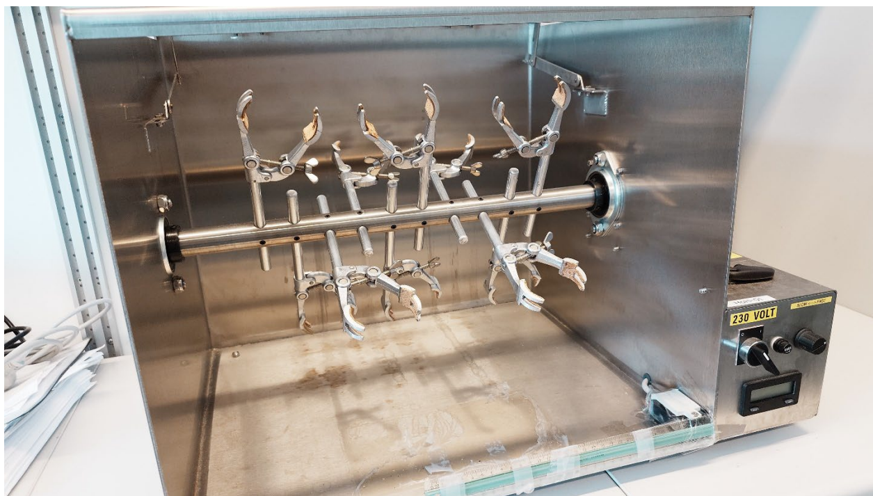
Figure 6: Overhead shaker used for equilibrium experiments.
