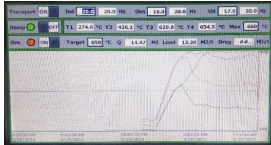
Figure 2: Temperature/time diagram of the production of the wood-biochar at AquaGreen.
