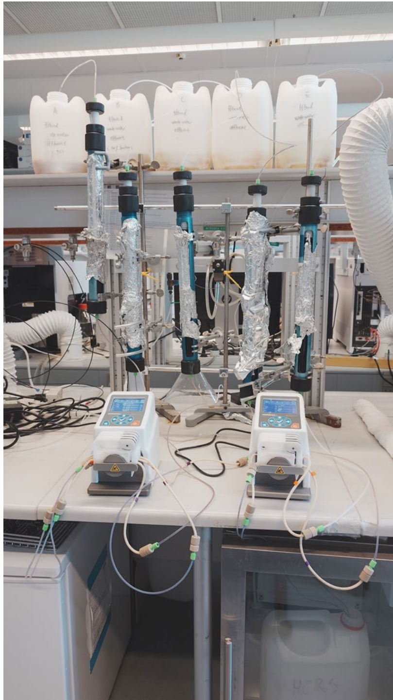
Figure 5: Experimental setup for the micropollutant column experiment.
